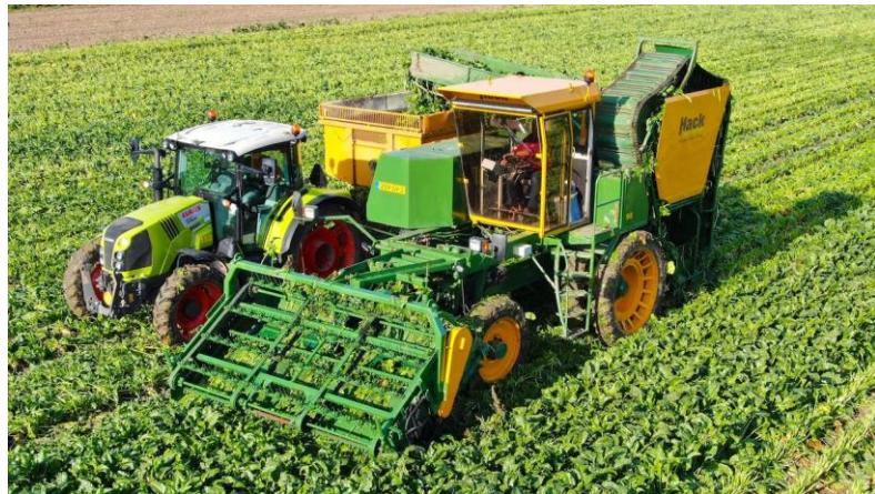
The Hack harvester designed for sugar beet leaves harvest is actually a modified spinach harvester.
